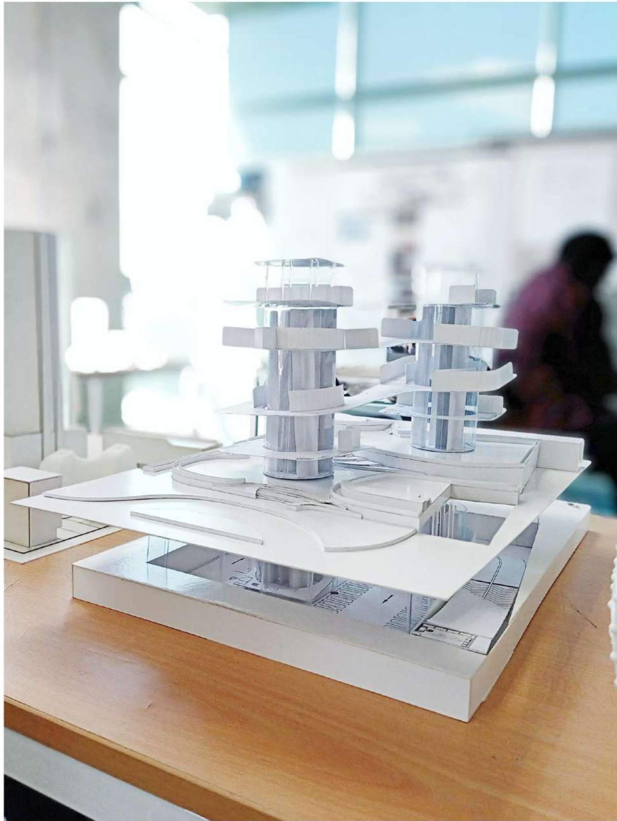
A blow-up physical model (w/out facade) to understand spatial relationships & circulations.
